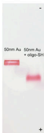
Figure 1. 0.5% (w/v) agarose gel analysis of 50nm OligoREADY™ gold nanoparticles before and after functionalization with a thiolated oligonucleotide (20 bases). Gel was operated at 100V in 0.5X TBE buffer for 30 minutes.
